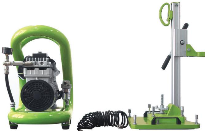
3, Connect vacuum pump with vacuum pad through vacuum hose.
